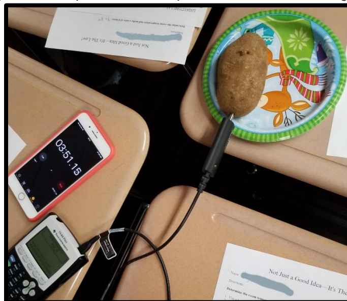
Picture #5: Students recorded the temperature of a baked potato in five-minute intervals. They also noted the room temperature so they could apply Newton's Law of Cooling.
