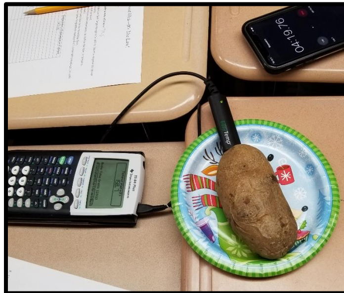
Picture #4: Students gathered temperature data on their baked potato. The Vernier EasyTemp constantly displayed the temperature of the potato on the TI-84 Plus graphing calculator.
